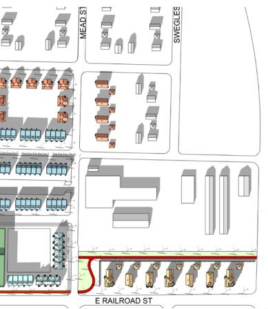
Vehicular access for housing along the trail is located behind housing via an alley, limiting vehicular crossing of the trailway to street intersections and reducing pedestrian and vehicle interaction points. This retains the separated nature of the trail and improves safety.
