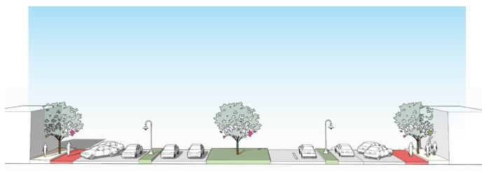
A variation on the three-lane configuration of concept 1, with non-motorized facilities moved to the edges of the ROW, immediately next to storefronts.
